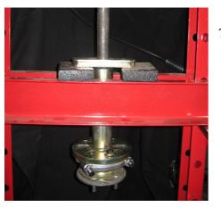
7. Remove seals and bearing out of the backing plate and Hub and reassemble as per Vehicle makers instructions.
